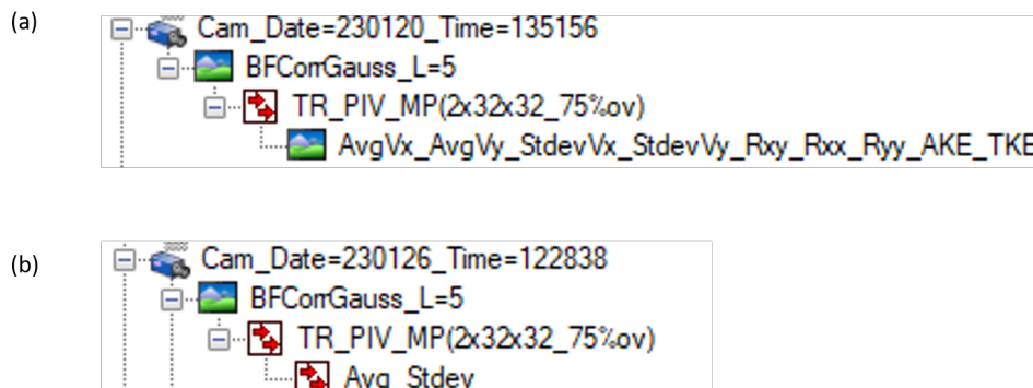
Figure 15: Available processed data if (a) the vector statistics results (see Figure 12 are set properly and (b) if the vector statistics results are set improperly
