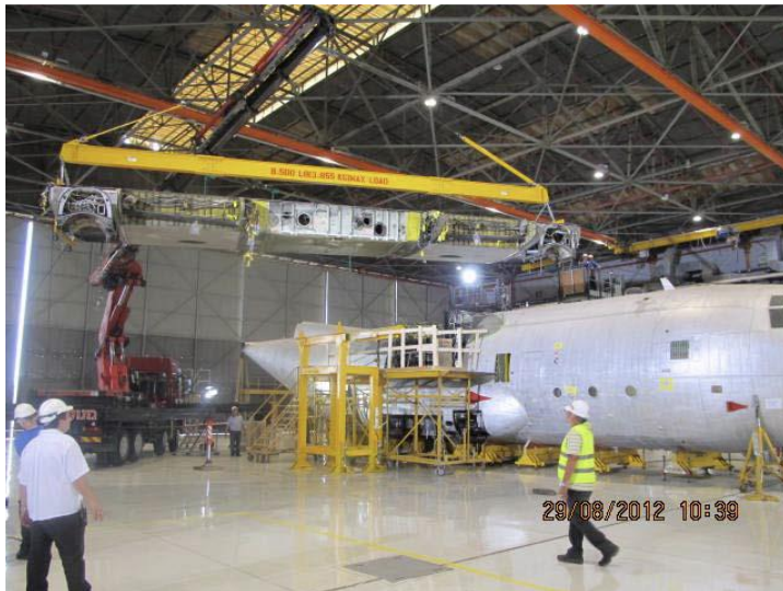
Source: Strul, E., "IAI C-130 Life Extension Program CWB Replacement," C-130 Hercules Operators Council, 2013
