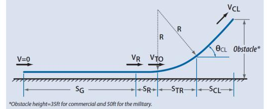
For low take-off distance, it's good to have HIGH values of maximum lift coefficient, C<sub>Lmax</sub>; thrust-to-weight ratio, T/W; and air density (lower altitudes)...but beware of the downsides!
